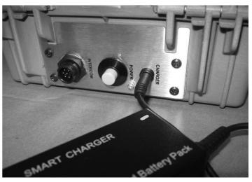
To turn the ComHub on, press the Yellow Power Button and the Power LED will light up (see ComHub Exterior Control Panel & Connections).
